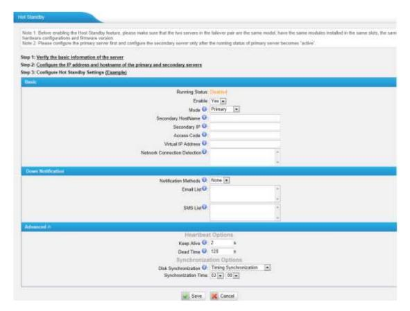
Figure 5-20 Hot Standby Configuration
