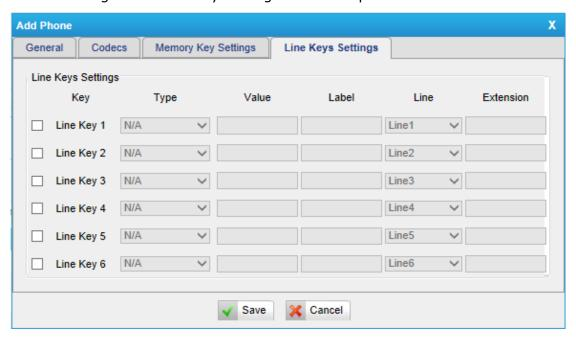
Figure 6-16 Configure Line Key
