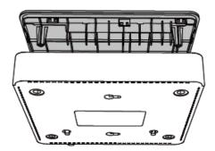
STEP 2 Insert the module to the Module Slot.
