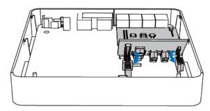
**STEP 3** Insert a SIM card on the GSM/3G module following the instructions. Skip this step if no GSM/3G module installed.
